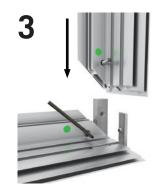
Once in place, tighten **set screws** with allen wrench on **L angle corners**, just enough to catch. Re-insert **HD screws** into the **HD corners** and loosely tighten with allen wrench, just enough to catch. Repeat until all corners of the frame are loosely assembled.
