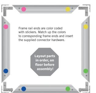
Loosen set screws on all L angle corners so they can become flush. Remove HD corner bracket screws from each of the HD corner brackets with supplied allen wrench—set aside.
