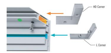
**6** Once in place, tighten **set screws** with Allen wrench on **L Corners** just enough to catch. Re-insert **HD screws** into the **HD Corner** and loosely tighten with Allen wrench just enough to catch. Repeat until all corners of the frame are loosely assembled.
