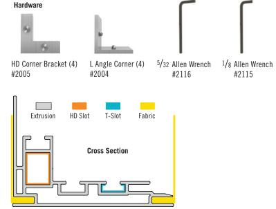
2 Start by assembling one corner of the frame at a time. Insert an **L angle corner** into the rail's **T-slot** (highlighted in blue). Insert an **HD corner bracket** into the rail's **HD slot** (highlighted in orange).
